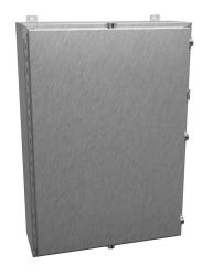
Hammond enclosure, NEMA 3R/4/4X/12/13, 42 x 30 x 10in (HxWxD), wall mount, 304 stainless steel, #4 brush finish, single-door, stainless steel clamps, padlock hasp and staple.
