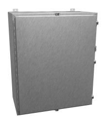
Hammond enclosure, NEMA 3R/4/4X/12/13, 36 x 30 x 16in (HxWxD), wall mount, 304 stainless steel, #4 brush finish, single-door, stainless steel clamps, padlock hasp and staple.
