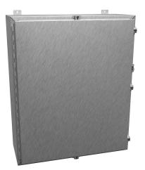
Hammond enclosure, NEMA 3R/4/4X/12/13, 36 x 30 x 12in (HxWxD), wall mount, 304 stainless steel, #4 brush finish, single-door, stainless steel clamps, padlock hasp and staple.
