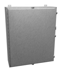
Hammond enclosure, NEMA 3R/4/4X/12/13, 36 x 30 x 10in (HxWxD), wall mount, 304 stainless steel, #4 brush finish, single-door, stainless steel clamps, padlock hasp and staple.
