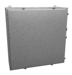
Hammond enclosure, NEMA 3R/4/4X/12/13, 36 x 36 x 12in (HxWxD), wall mount, 304 stainless steel, #4 brush finish, single-door, stainless steel clamps, padlock hasp and staple.
