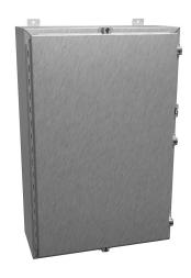
Hammond enclosure, NEMA 3R/4/4X/12/13, 36 x 24 x 10in (HxWxD), wall mount, 304 stainless steel, #4 brush finish, single-door, stainless steel clamps, padlock hasp and staple.
