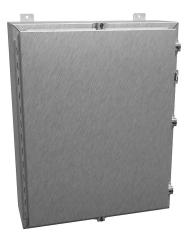
Hammond enclosure, NEMA 3R/4/4X/12/13, 30 x 24 x 8in (HxWxD), wall mount, 304 stainless steel, #4 brush finish, single-door, stainless steel clamps, padlock hasp and staple.
