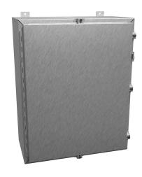
Hammond enclosure, NEMA 3R/4/4X/12/13, 30 x 24 x 12in (HxWxD), wall mount, 304 stainless steel, #4 brush finish, single-door, stainless steel clamps, padlock hasp and staple.
