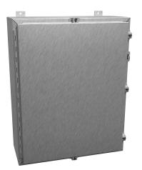
Hammond enclosure, NEMA 3R/4/4X/12/13, 30 x 24 x 10in (HxWxD), wall mount, 304 stainless steel, #4 brush finish, single-door, stainless steel clamps, padlock hasp and staple.
