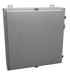
Hammond enclosure, NEMA 3R/4/4X/12/13, 24 x 24 x 6in (HxWxD), wall mount, 304 stainless steel, #4 brush finish, single-door, stainless steel clamps, padlock hasp and staple.
