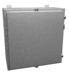
Hammond enclosure, NEMA 3R/4/4X/12/13, 24 x 24 x 12in (HxWxD), wall mount, 304 stainless steel, #4 brush finish, single-door, stainless steel clamps, padlock hasp and staple.
