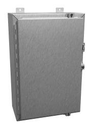
Hammond enclosure, NEMA 3R/4/4X/12/13, 24 x 16 x 8in (HxWxD), wall mount, 304 stainless steel, #4 brush finish, single-door, stainless steel clamps, padlock hasp and staple.
