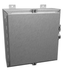
Hammond enclosure, NEMA 3R/4/4X/12/13, 16 x 16 x 6in (HxWxD), wall mount, 304 stainless steel, #4 brush finish, single-door, stainless steel clamps, padlock hasp and staple.
