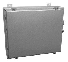
Hammond enclosure, NEMA 3R/4/4X/12/13, 20 x 24 x 8in (HxWxD), wall mount, 304 stainless steel, #4 brush finish, single-door, stainless steel clamps, padlock hasp and staple.
