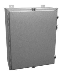
Hammond enclosure, NEMA 3R/4/4X/12/13, 24 x 20 x 8in (HxWxD), wall mount, 304 stainless steel, #4 brush finish, single-door, stainless steel clamps, padlock hasp and staple.
