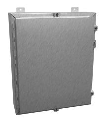
Hammond enclosure, NEMA 3R/4/4X/12/13, 24 x 20 x 6in (HxWxD), wall mount, 304 stainless steel, #4 brush finish, single-door, stainless steel clamps, padlock hasp and staple.
