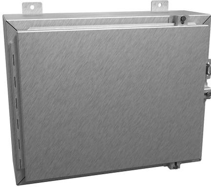
Hammond enclosure, NEMA 3R/4/4X/12/13, 16 x 20 x 6in (HxWxD), wall mount, 304 stainless steel, #4 brush finish, single-door, stainless steel clamps, padlock hasp and staple.
