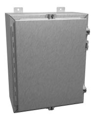
Hammond enclosure, NEMA 3R/4/4X/12/13, 20 x 16 x 8in (HxWxD), wall mount, 304 stainless steel, #4 brush finish, single-door, stainless steel clamps, padlock hasp and staple.
