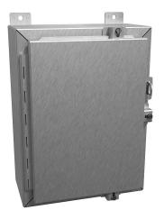
Hammond enclosure, NEMA 3R/4/4X/12/13, 16 x 12 x 6in (HxWxD), wall mount, 304 stainless steel, #4 brush finish, single-door, stainless steel clamps, padlock hasp and staple.
