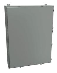
Hammond enclosure, NEMA 3R/4/12, 48 x 36 x 8in (HxWxD), wall mount, carbon steel, ANSI 61 gray, powder coat finish, single-door, stainless steel clamps, padlock hasp and staple.
