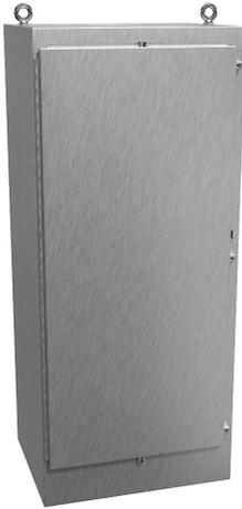
Hammond enclosure, NEMA 3R/4/4X/12/13, 72 x 30 x 24in (HxWxD), freestanding, 316 stainless steel, #4 brush finish, single-door, stainless steel clamps, padlock hasp and staple.
