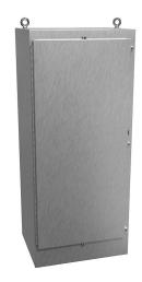
Hammond enclosure, NEMA 3R/4/4X/12/13,  $72 \times 30 \times 24$ in (HxWxD), freestanding, 316 stainless steel, #4 brush finish, singledoor, stainless steel clamps, padlock hasp and staple.
