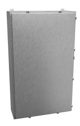
Hammond enclosure, NEMA 3R/4/4X/12/13, 60 x 36 x 12in (HxWxD), wall mount, 316 stainless steel, #4 brush finish, single-door, stainless steel clamps, padlock hasp and staple.
