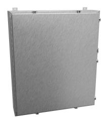
Hammond enclosure, NEMA 3R/4/4X/12/13, 42 x 36 x 8in (HxWxD), wall mount, 316 stainless steel, #4 brush finish, single-door, stainless steel clamps, padlock hasp and staple.
