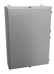
Hammond enclosure, NEMA 3R/4/4X/12/13, 42 x 30 x 10in (HxWxD), wall mount, 316 stainless steel, #4 brush finish, single-door, stainless steel clamps, padlock hasp and staple.
