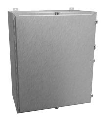
Hammond enclosure, NEMA 3R/4/4X/12/13, 36 x 30 x 16in (HxWxD), wall mount, 316 stainless steel, #4 brush finish, single-door, stainless steel clamps, padlock hasp and staple.
