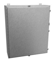
Hammond enclosure, NEMA 3R/4/4X/12/13, 36 x 30 x 10in (HxWxD), wall mount, 316 stainless steel, #4 brush finish, singledoor, stainless steel clamps, padlock hasp and staple.
