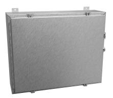
Hammond enclosure, NEMA 3R/4/4X/12/13, 24 x 30 x 8in (HxWxD), wall mount, 316 stainless steel, #4 brush finish, single-door, stainless steel clamps, padlock hasp and staple.
