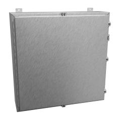
Hammond enclosure, NEMA 3R/4/4X/12/13, 30 x 30 x 8in (HxWxD), wall mount, 316 stainless steel, #4 brush finish, single-door, stainless steel clamps, padlock hasp and staple.
