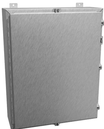
Hammond enclosure, NEMA 3R/4/4X/12/13, 30 x 24 x 8in (HxWxD), wall mount, 316 stainless steel, #4 brush finish, single-door, stainless steel clamps, padlock hasp and staple.
