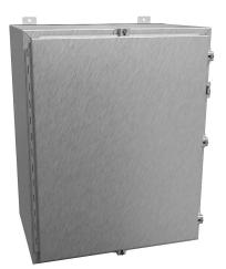
Hammond enclosure, NEMA 3R/4/4X/12/13, 30 x 24 x 16in (HxWxD), wall mount, 316 stainless steel, #4 brush finish, single-door, stainless steel clamps, padlock hasp and staple.
