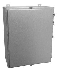
Hammond enclosure, NEMA 3R/4/4X/12/13, 30 x 24 x 12in (HxWxD), wall mount, 316 stainless steel, #4 brush finish, single-door, stainless steel clamps, padlock hasp and staple.
