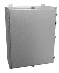
Hammond enclosure, NEMA 3R/4/4X/12/13, 30 x 24 x 10in (HxWxD), wall mount, 316 stainless steel, #4 brush finish, single-door, stainless steel clamps, padlock hasp and staple.
