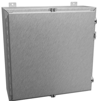
Hammond enclosure, NEMA 3R/4/4X/12/13, 24 x 24 x 8in (HxWxD), wall mount, 316 stainless steel, #4 brush finish, single-door, stainless steel clamps, padlock hasp and staple.
