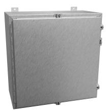
Hammond enclosure, NEMA 3R/4/4X/12/13, 24 x 24 x 12in (HxWxD), wall mount, 316 stainless steel, #4 brush finish, single-door, stainless steel clamps, padlock hasp and staple.
