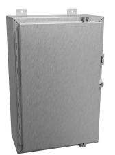
Hammond enclosure, NEMA 3R/4/4X/12/13, 24 x 16 x 8in (HxWxD), wall mount, 316 stainless steel, #4 brush finish, single-door, stainless steel clamps, padlock hasp and staple.
