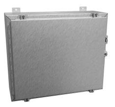
Hammond enclosure, NEMA 3R/4/4X/12/13, 20 x 24 x 8in (HxWxD), wall mount, 316 stainless steel, #4 brush finish, single-door, stainless steel clamps, padlock hasp and staple.
