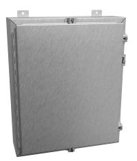
Hammond enclosure, NEMA 3R/4/4X/12/13, 24 x 20 x 6in (HxWxD), wall mount, 316 stainless steel, #4 brush finish, single-door, stainless steel clamps, padlock hasp and staple.
