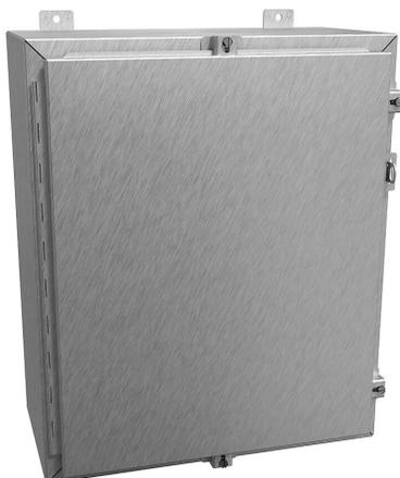
Hammond enclosure, NEMA 3R/4/4X/12/13, 24 x 20 x 10in (HxWxD), wall mount, 316 stainless steel, #4 brush finish, single-door, stainless steel clamps, padlock hasp and staple.
