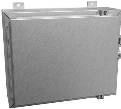
Hammond enclosure, NEMA 3R/4/4X/12/13, 16 x 20 x 6in (HxWxD), wall mount, 316 stainless steel, #4 brush finish, single-door, stainless steel clamps, padlock hasp and staple.
