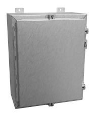
Hammond enclosure, NEMA 3R/4/4X/12/13, 20 x 16 x 8in (HxWxD), wall mount, 316 stainless steel, #4 brush finish, single-door, stainless steel clamps, padlock hasp and staple.
