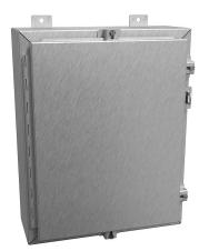
Hammond enclosure, NEMA 3R/4/4X/12/13, 20 x 16 x 6in (HxWxD), wall mount, 316 stainless steel, #4 brush finish, single-door, stainless steel clamps, padlock hasp and staple.
