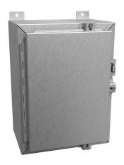
Hammond enclosure, NEMA 3R/4/4X/12/13, 16 x 12 x 8in (HxWxD), wall mount, 316 stainless steel, #4 brush finish, single-door, stainless steel clamps, padlock hasp and staple.
