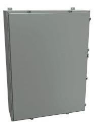
Hammond enclosure, NEMA 3R/4/12, 48 x 36 x 12in (HxWxD), wall mount, carbon steel, ANSI 61 gray, powder coat finish, single-door, stainless steel clamps, padlock hasp and staple.
