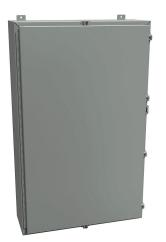
Hammond enclosure, NEMA 3R/4/12, 48 x 30 x 10in (HxWxD), wall mount, carbon steel, ANSI 61 gray, powder coat finish, single-door, stainless steel clamps, padlock hasp and staple.
