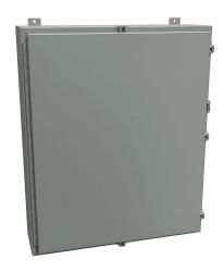
Hammond enclosure, NEMA 3R/4/12, 36 x 30 x 8in (HxWxD), wall mount, carbon steel, ANSI 61 gray, powder coat finish, single-door, stainless steel clamps, padlock hasp and staple.
