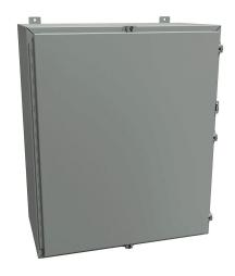
Hammond enclosure, NEMA 3R/4/12,  $36 \times 30 \times 16$ in (HxWxD), wall mount, carbon steel, ANSI 61 gray, powder coat finish, single-door, stainless steel clamps, padlock hasp and staple.
