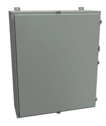
Hammond enclosure, NEMA 3R/4/12, 36 x 30 x 10in (HxWxD), wall mount, carbon steel, ANSI 61 gray, powder coat finish, single-door, stainless steel clamps, padlock hasp and staple.
