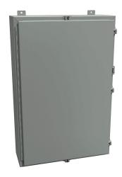
Hammond enclosure, NEMA 3R/4/12, 36 x 24 x 8in (HxWxD), wall mount, carbon steel, ANSI 61 gray, powder coat finish, single-door, stainless steel clamps, padlock hasp and staple.
