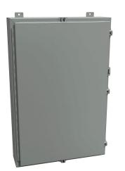
Hammond enclosure, NEMA 3R/4/12, 36 x 24 x 6in (HxWxD), wall mount, carbon steel, ANSI 61 gray, powder coat finish, single-door, stainless steel clamps, padlock hasp and staple.
