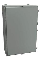
Hammond enclosure, NEMA 3R/4/12, 36 x 24 x 12in (HxWxD), wall mount, carbon steel, ANSI 61 gray, powder coat finish, single-door, stainless steel clamps, padlock hasp and staple.
